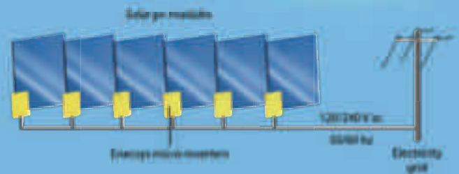
Advanced solar PV system using Enecsys solar micro-inverters avoids the Domino Effect... enabling maximum energy harvest
